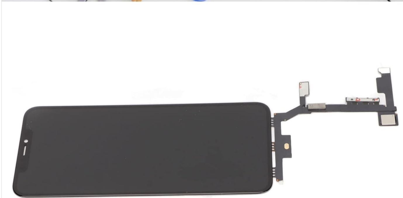
Image 5.2: A close-up view of the flex cables and connectors on the back of an iPhone screen, highlighting the intricate connections that need to be handled during component transfer.
