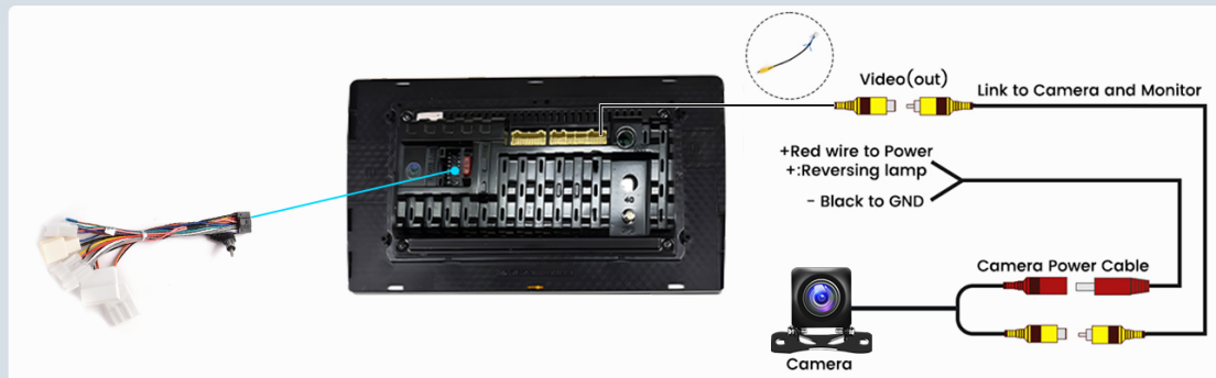
Image 3.2: Detailed wiring diagram for connecting the backup camera.
