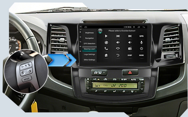
Image 3.3: Interface for configuring steering wheel controls.
