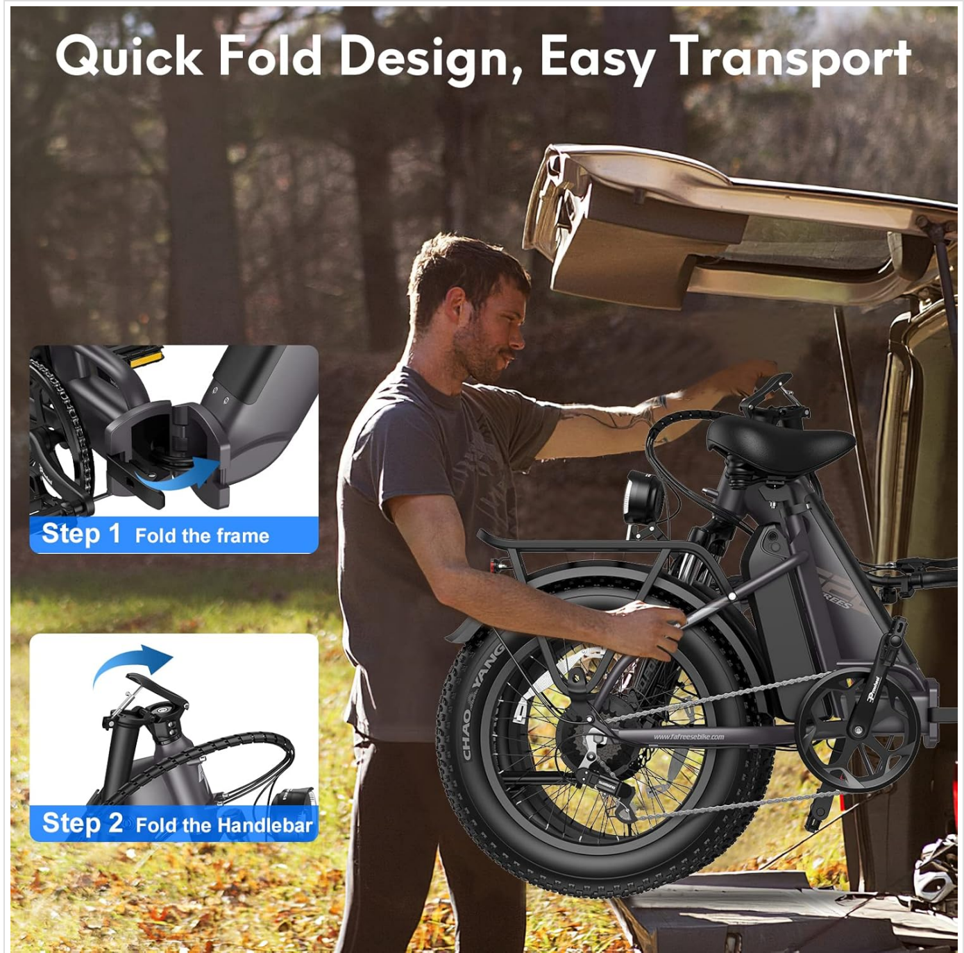
Figure 4.2: Visual guide demonstrating the two main steps for folding the Fafrees FF20 electric fatbike: folding the frame and folding the handlebar, making it easy to transport.
