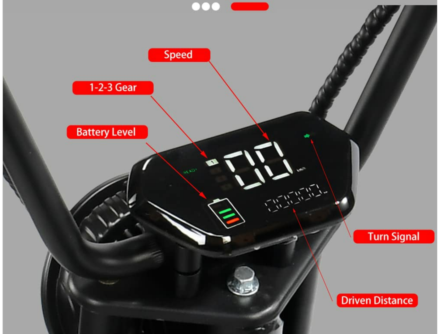
Figure 5.1: The LCD display panel, indicating current speed, battery level, selected gear (1-2-3), turn signal status, and driven distance.
