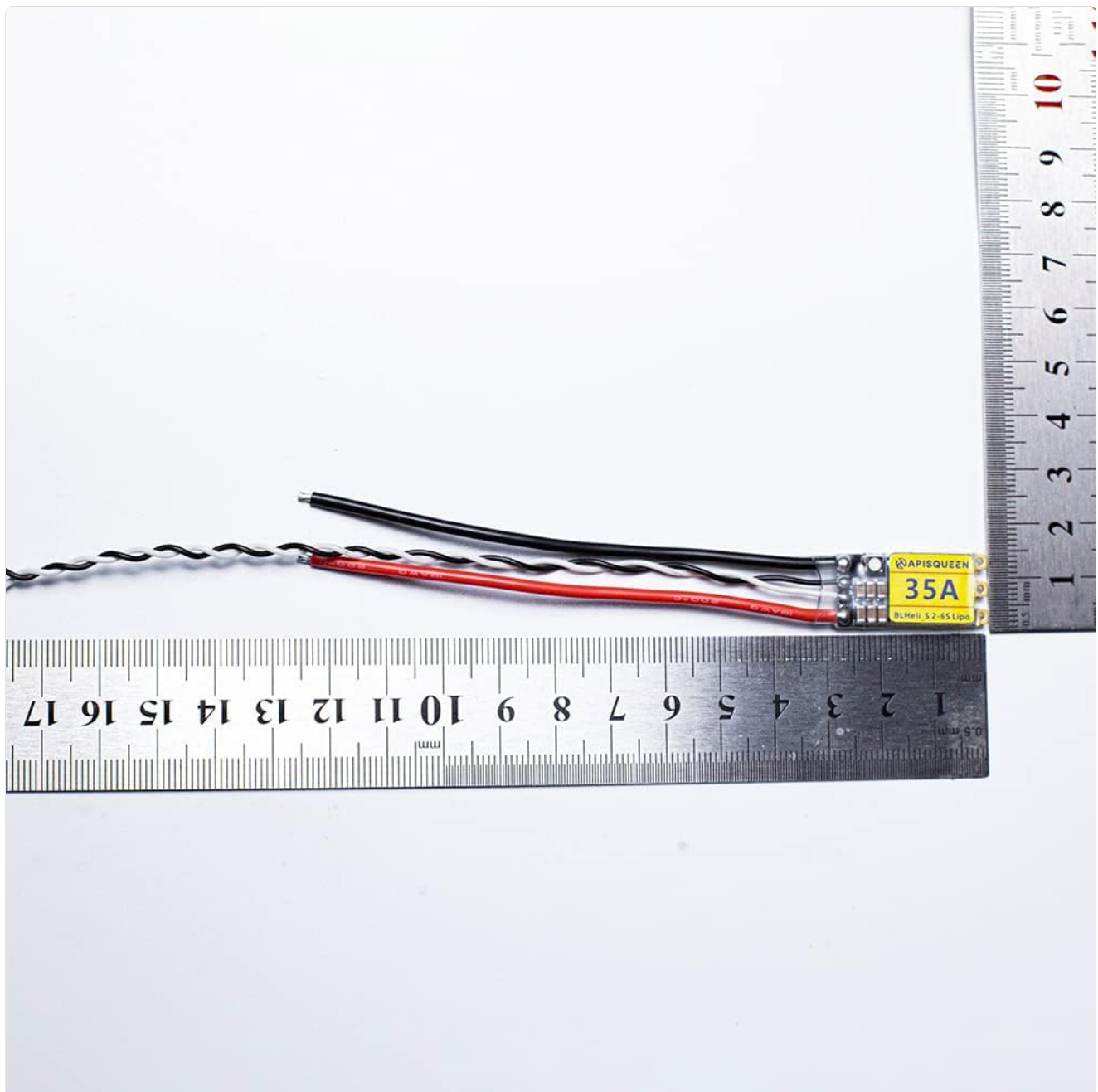
Figure 9.1: An ApisQueen 35A BLHeli_S ESC positioned alongside a ruler, illustrating its compact dimensions for easy integration into various drone builds.
