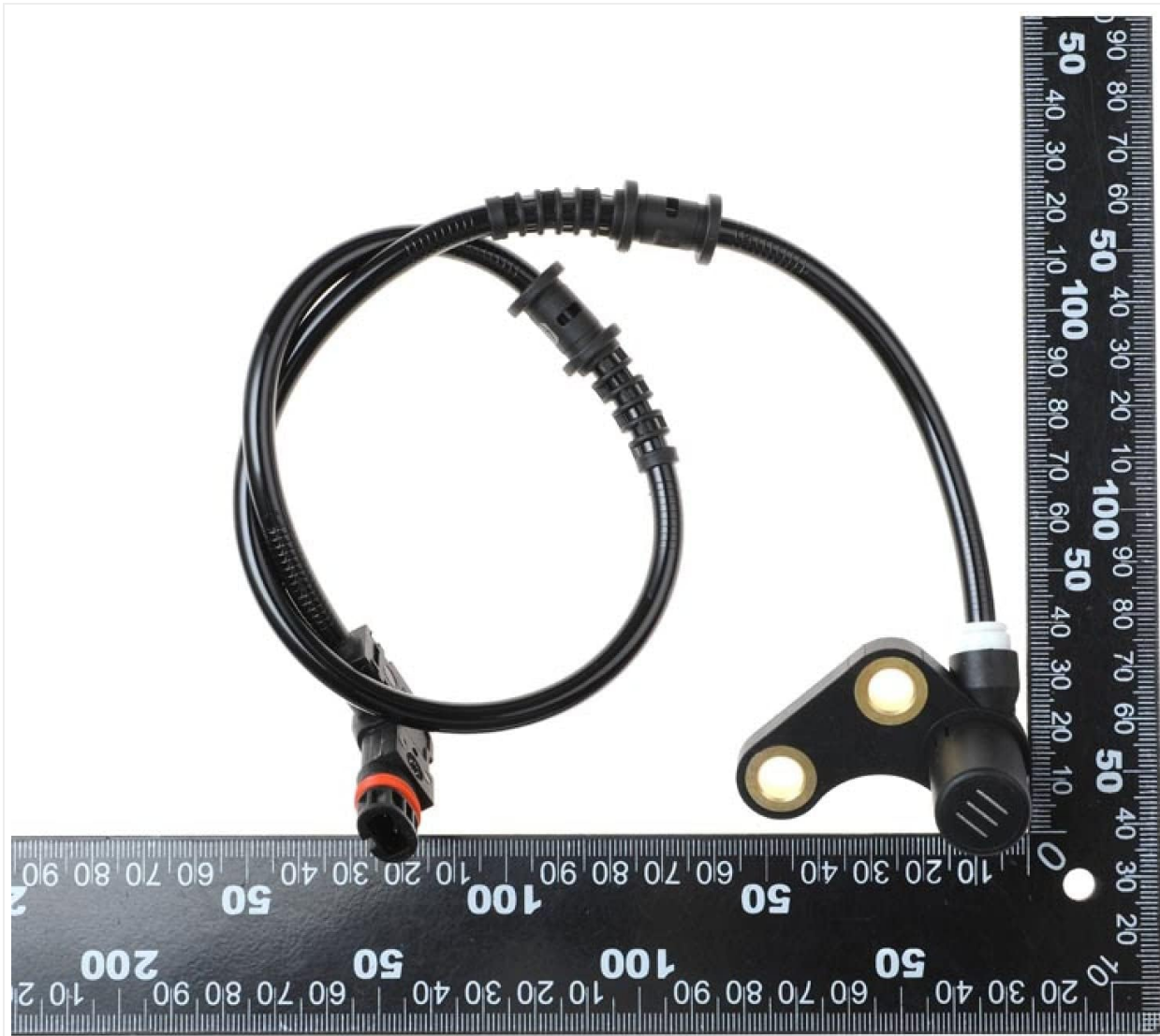
Figure 5: Sensor dimensions for reference.
