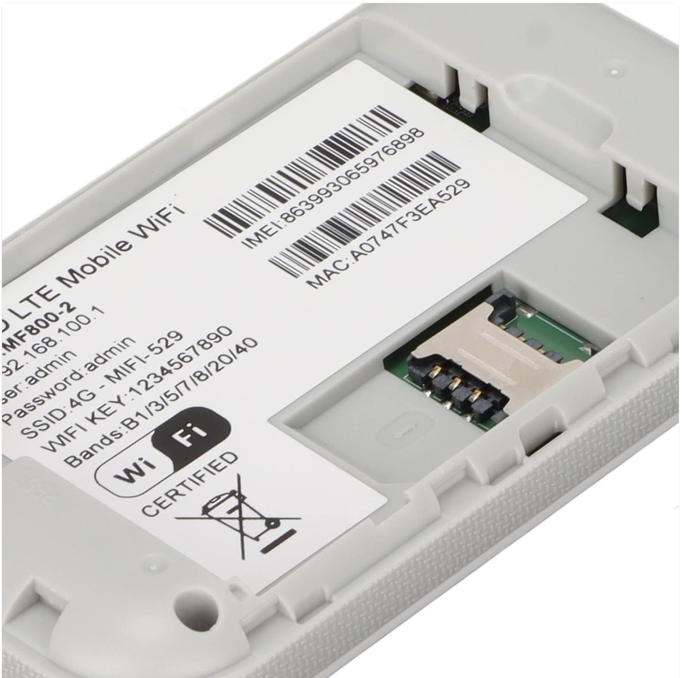
Figure 3: Close-up view of the SIM card slot and the product label displaying default Wi-Fi credentials.
