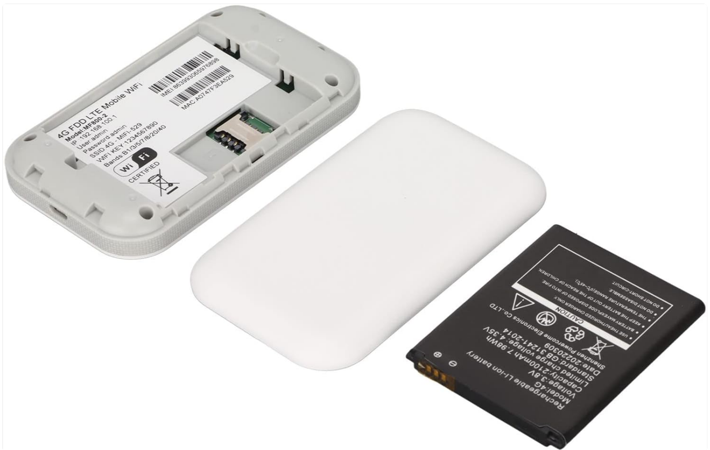
Figure 2: The router with its back cover removed, showing the battery and SIM card slot.
