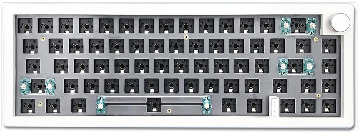
Figure 1: BOYI GMK67 Barebones Keyboard Kit, showing the layout without keycaps or switches.
