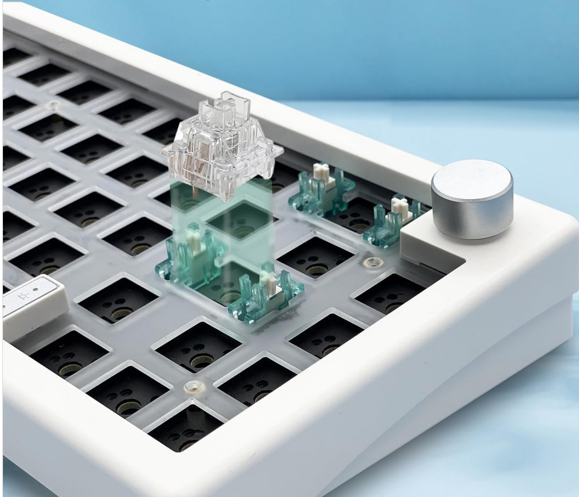
Figure 3: Demonstration of hot-swappable switch installation into the PCB.
