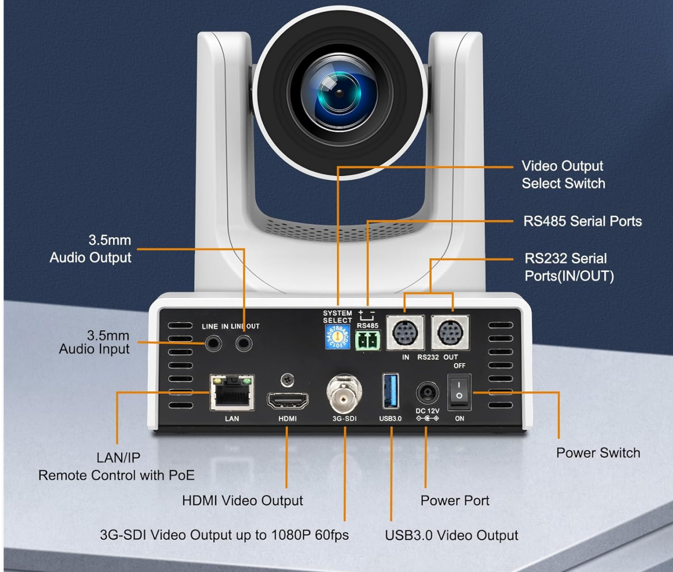
Figure 2: Detailed view of the camera's rear panel connectivity.
