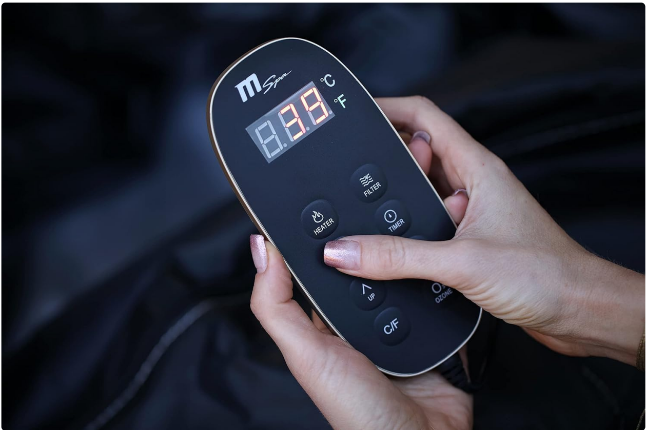
Image: The MSpa wired control panel, showing buttons for heater, bubble, filter, timer, and temperature adjustment.
