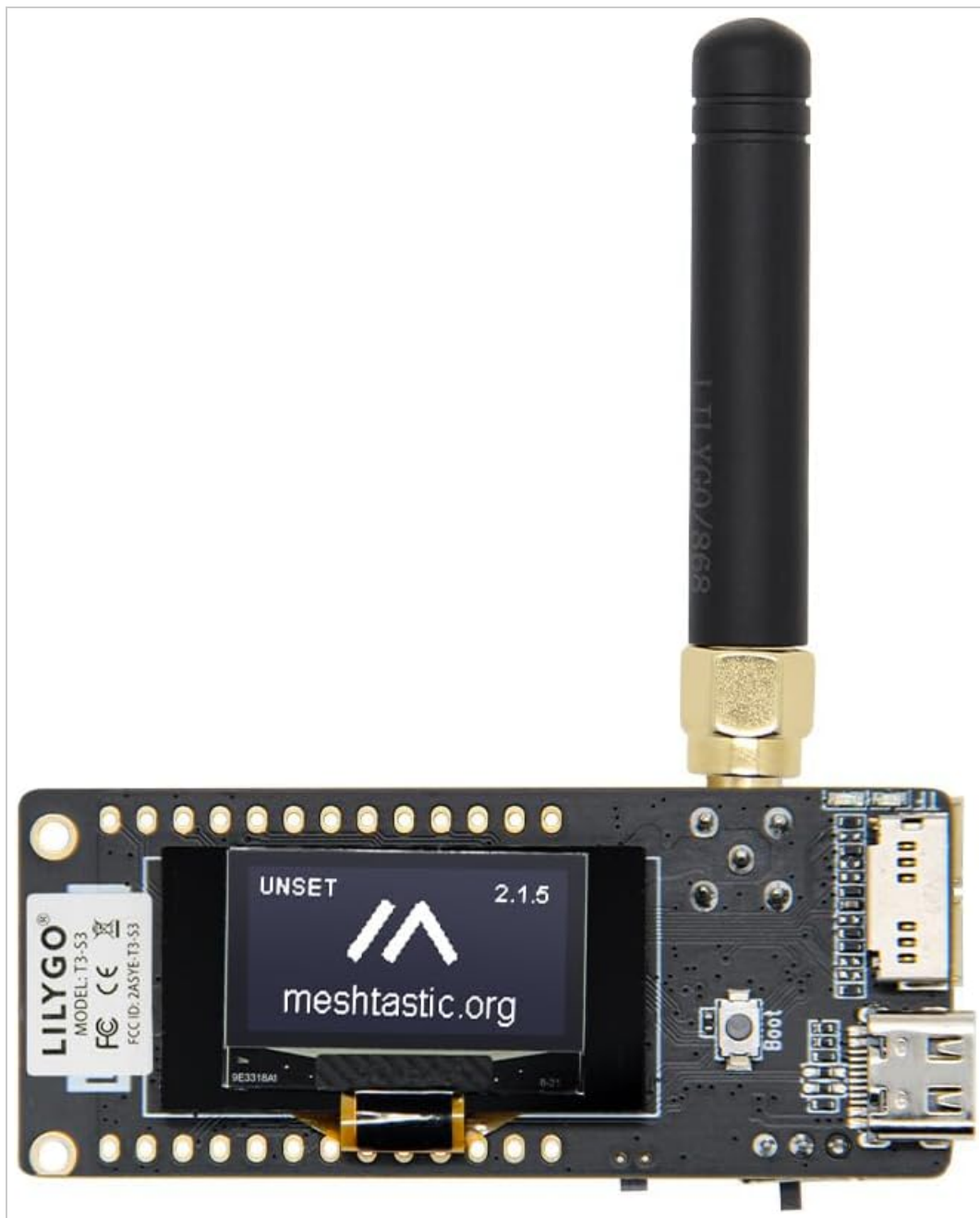
Figure 1: Front view of the LILYGO T3S3 ESP32-S3 LoRa Development Board, showing the integrated 0.96 inch OLED display.
