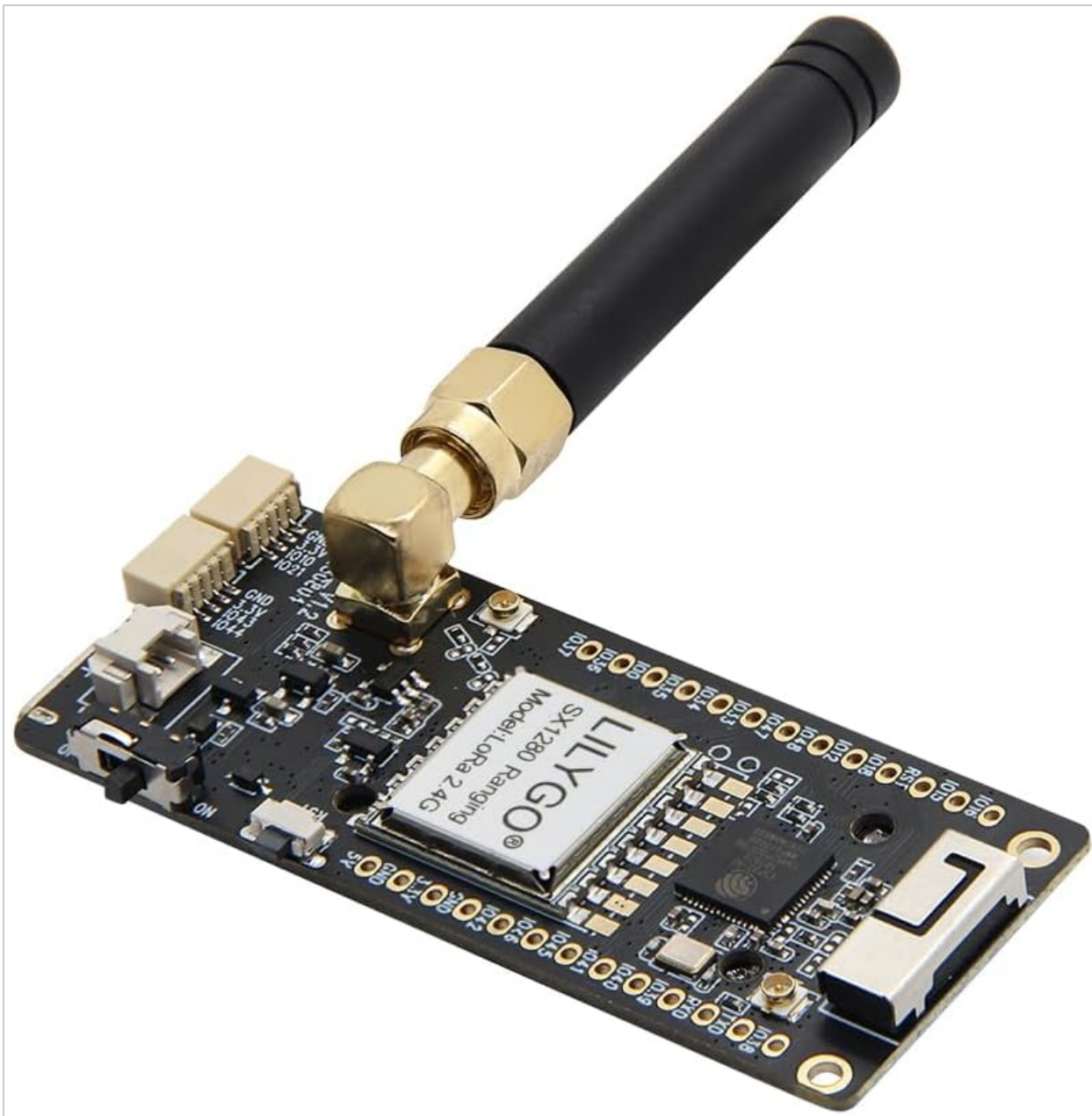
Figure 2: Back view of the LILYGO T3S3 ESP32-S3 LoRa Development Board, highlighting the LoRa module and other components.
