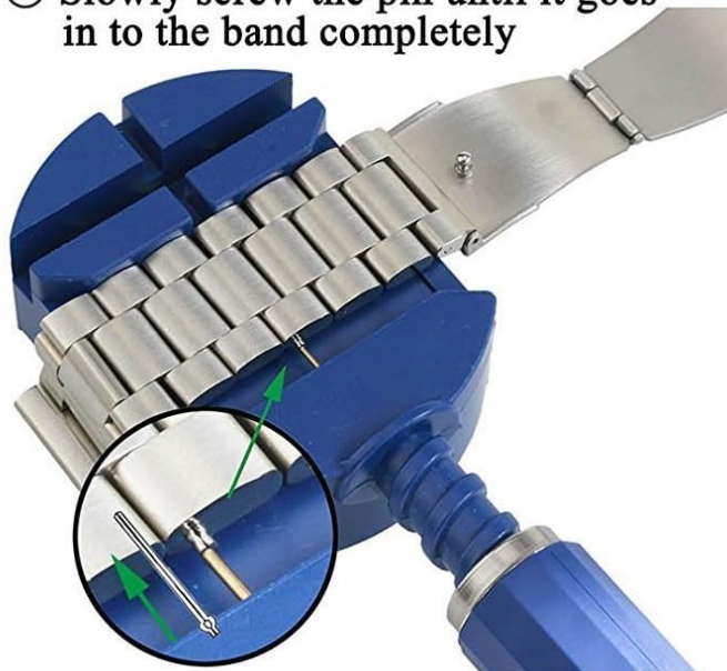
Figure 4: Detailed steps for using the link removal tool.
