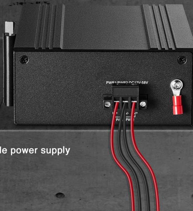
Figure 3.1: Illustration of the dual redundant power input design, highlighting the robust power connection terminals.
