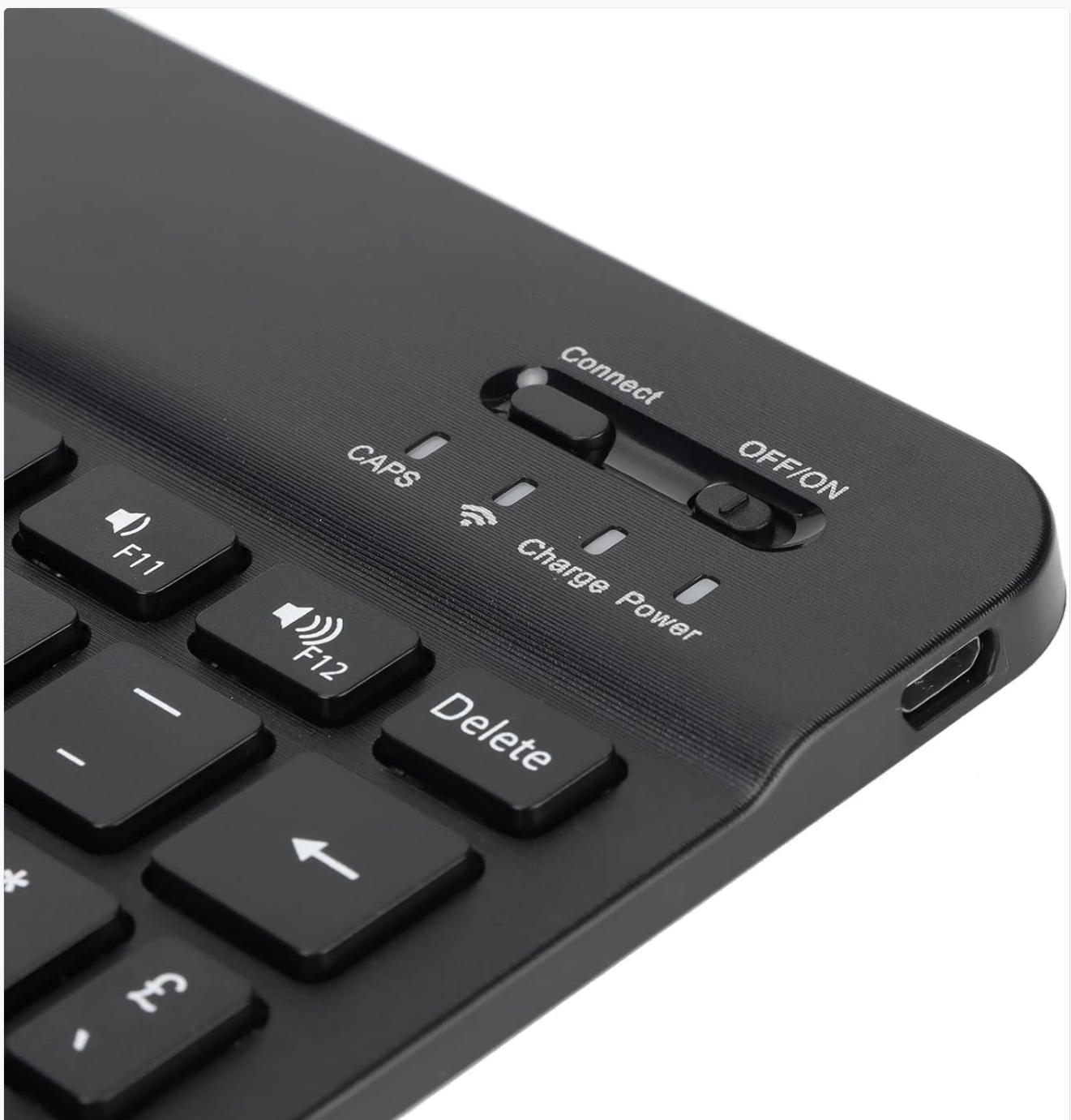
Image: A detailed view of the 'Connect' button and 'OFF/ON' switch on the top right of the keyboard, essential for initiating Bluetooth
