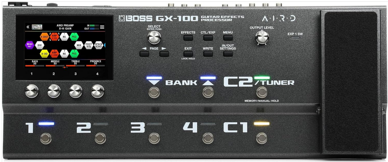
Image: Top view of the BOSS GX-100 Guitar Multi-effects Pedal, showcasing its footswitches, expression pedal, and color touchscreen display.
