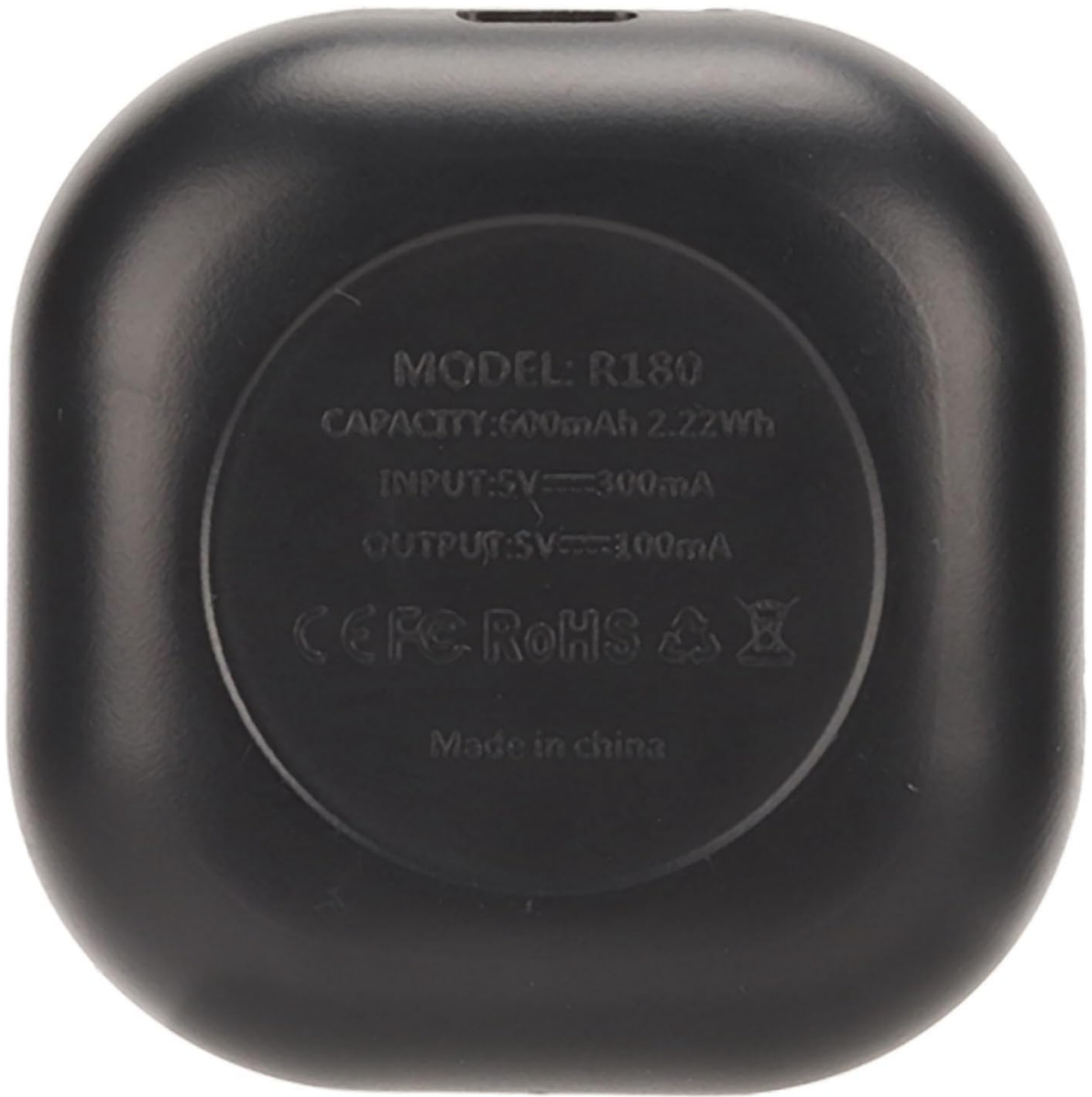
Figure 7.1: Bottom of the charging case displaying model and electrical information.
