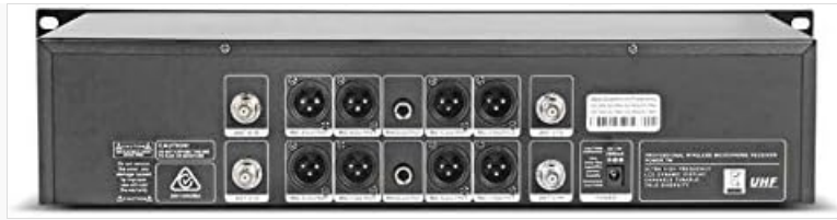
Image 4.1: Rear panel of the receiver, highlighting the XLR and 1/4" mixed audio output connections.
