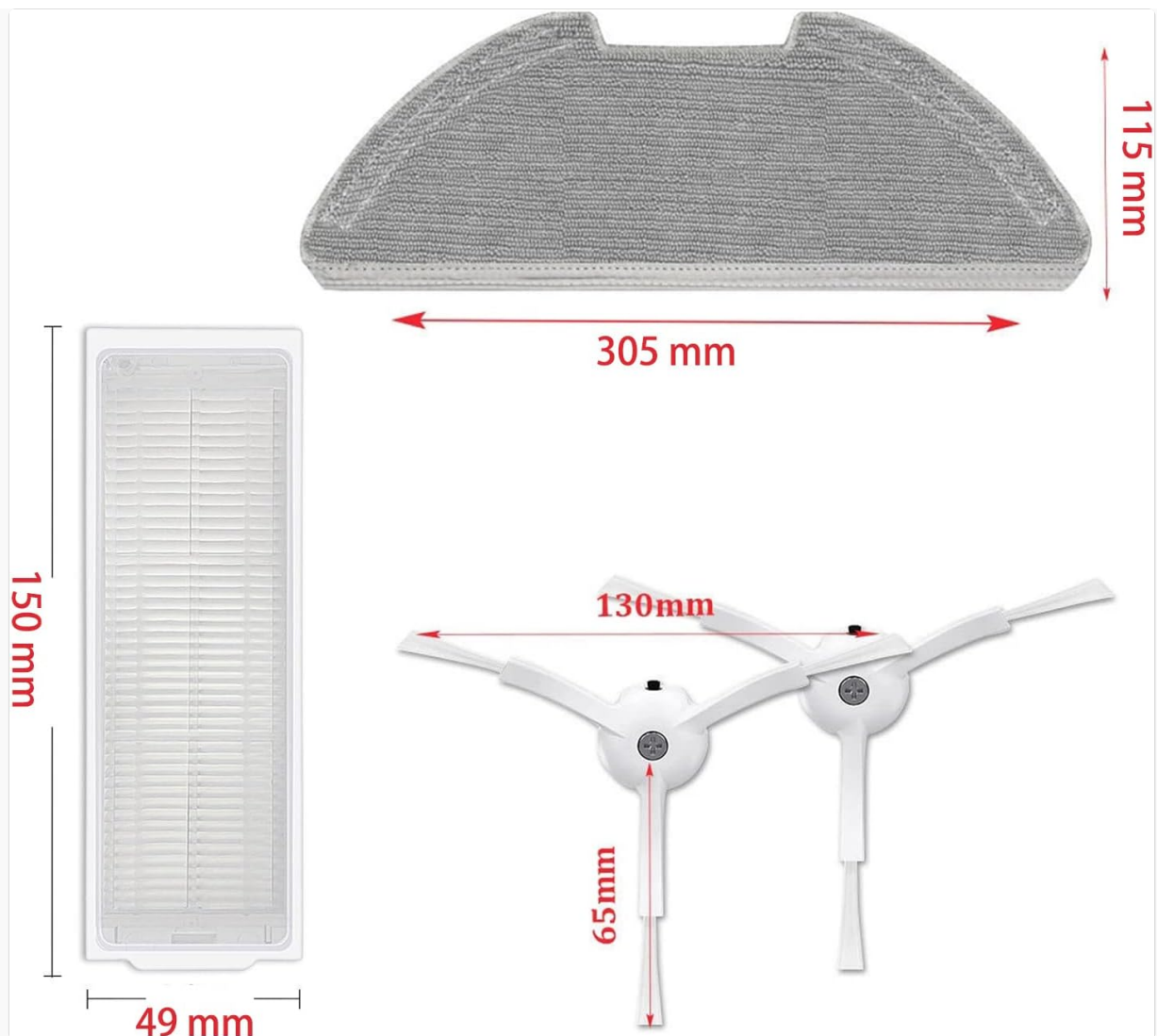
Image: An overview of the replacement kit components, including a mop pad (305mm x 115mm), a HEPA filter (150mm x 49mm), and two side brushes (130mm arm length, 65mm brush length).
