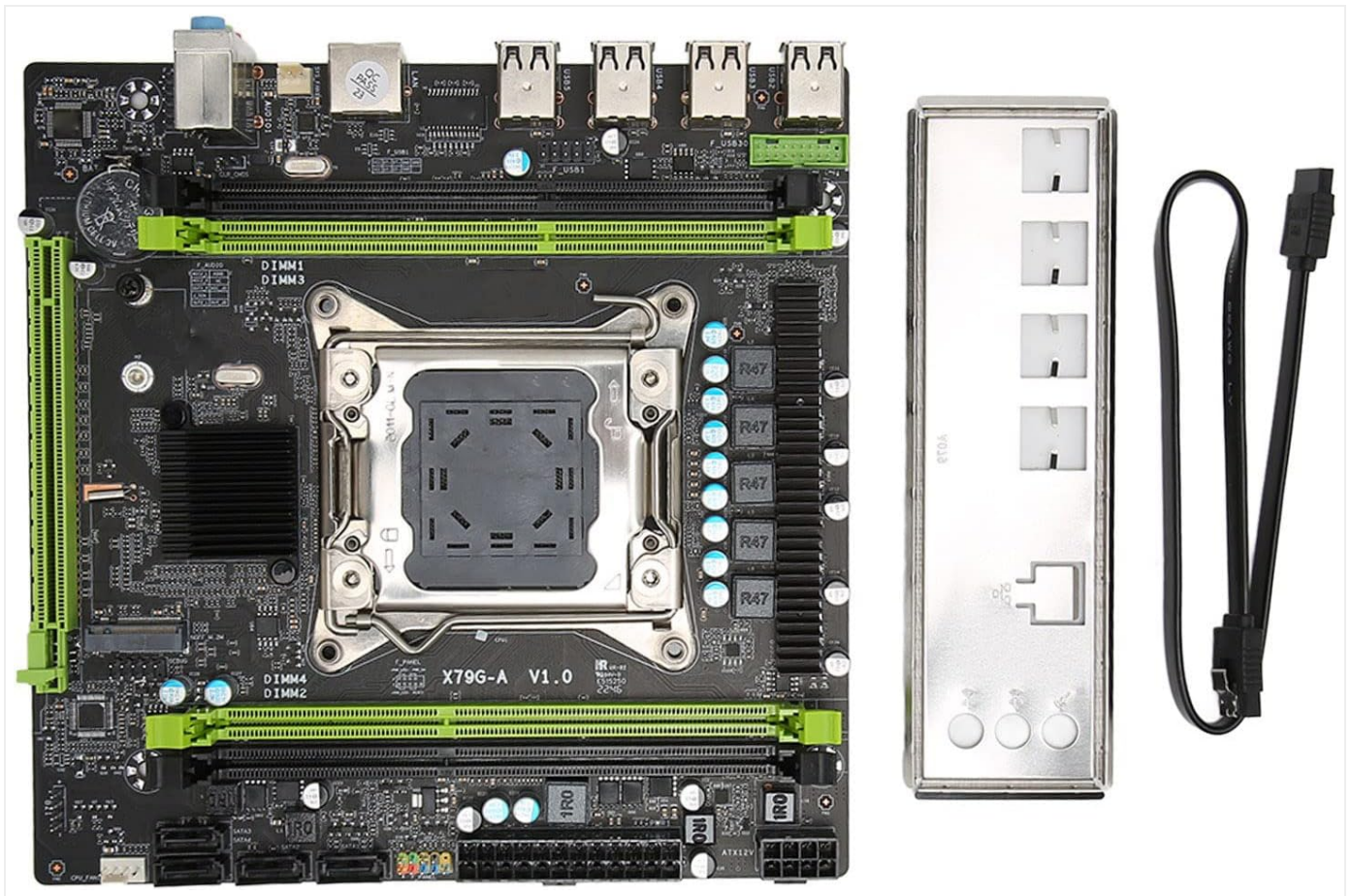
Figure 3.1: Mainboard and Accessories. This image shows the VBESTLIFE X79G A Mainboard alongside the included metal I/O shield and connection cable (SATA cable).
