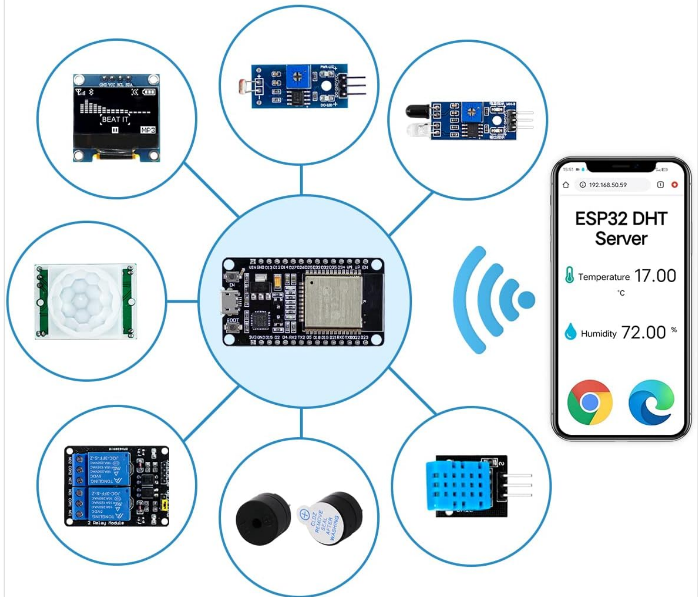
Figure 2.2: Diagram illustrating how the ESP32 board can wirelessly control and interact with various modules like OLED, DHT11, PIR sensor, and relay, often displaying data on a mobile device.
