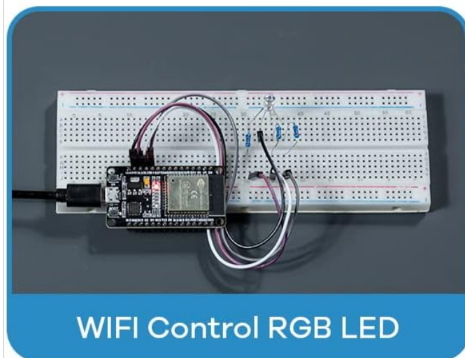
Figure 3.1: Examples of completed experiments on a breadboard, including ESP32 OLED Display, WiFi Monitor Temperature and Humidity, WiFi Control RGB LED, and WiFi Button Control Output.
