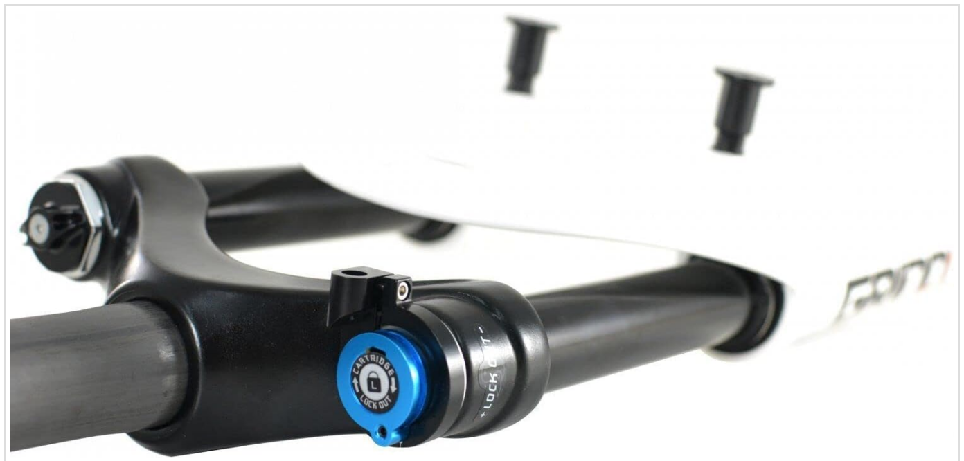
Figure 2.3: Detail of the remote lockout mechanism located on the fork crown, where the cable connects to engage or disengage the suspension.
