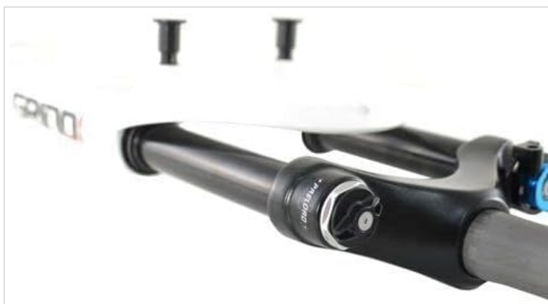
Figure 2.4: View of the preload adjustment knob, allowing riders to fine-tune the spring stiffness of the fork.
