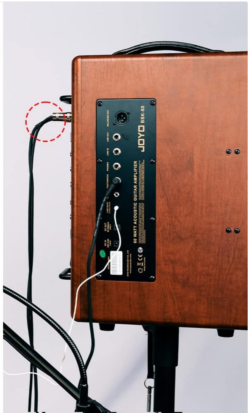
Image 4.2: The rubber protective shell reinforces the cable at the plug bend, preventing damage from repeated use.
