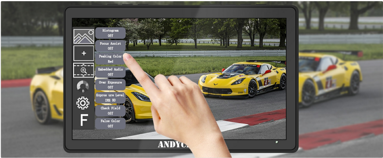
Image: A hand interacting with the touchscreen menu of the A6 Max, showing options like Histogram, Focus Assist, Peaking Color, and Exposure.
