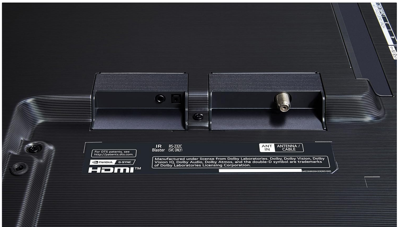
Image 4.2: A close-up view of the rear input panel of the LG G3 TV, showing connections for IR Blaster, RS-232C, and Antenna/Cable.
