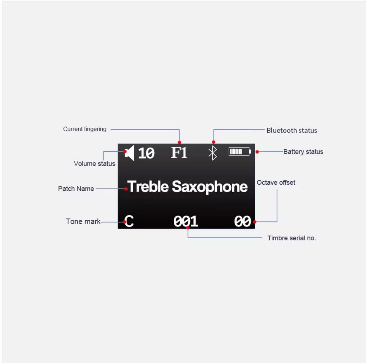
Figure 4.1: LCD display showing current fingering, volume status, patch name, tone mark, Bluetooth status, battery status, octave offset, and timbre serial number.
