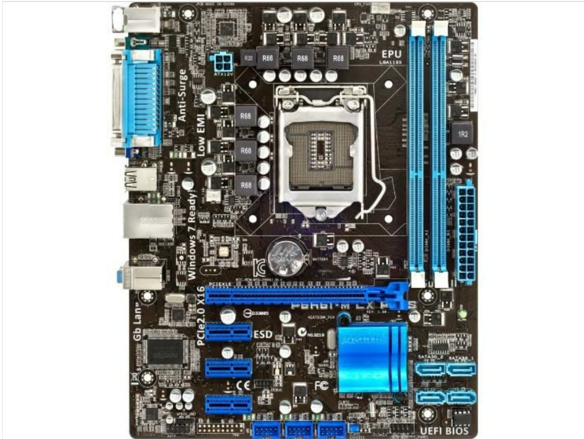
Figure 4.1: Motherboard Layout. This image displays the top-down view of the P8H61-M LX motherboard, highlighting key components such as the LGA 1155 CPU socket, two DDR3 DIMM slots, one PCIe 2.0 x16 slot, two PCIe x1 slots, four SATA ports, 24-pin ATX power connector, and 4-pin CPU power connector. Various headers for front panel connections are also visible.
