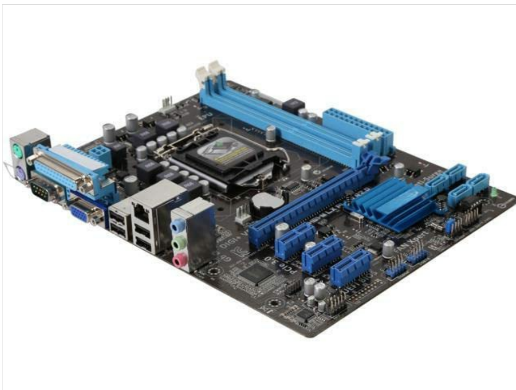
Figure 4.2: Angled Motherboard View. An angled perspective of the P8H61-M LX motherboard, providing a clearer view of the rear I/O panel and the overall component placement, including the chipsets heatsink and various onboard connectors.
