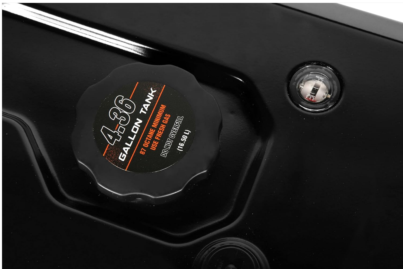
Image 4.2: A close-up of the fuel tank cap, indicating the 4.3-gallon capacity and recommended 87 octane minimum fuel.
