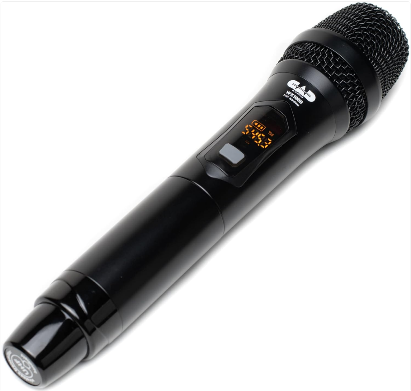
Image 5: Close-up of the CAD Audio WX1000HH handheld microphone's display, showing frequency and battery level indicators.
