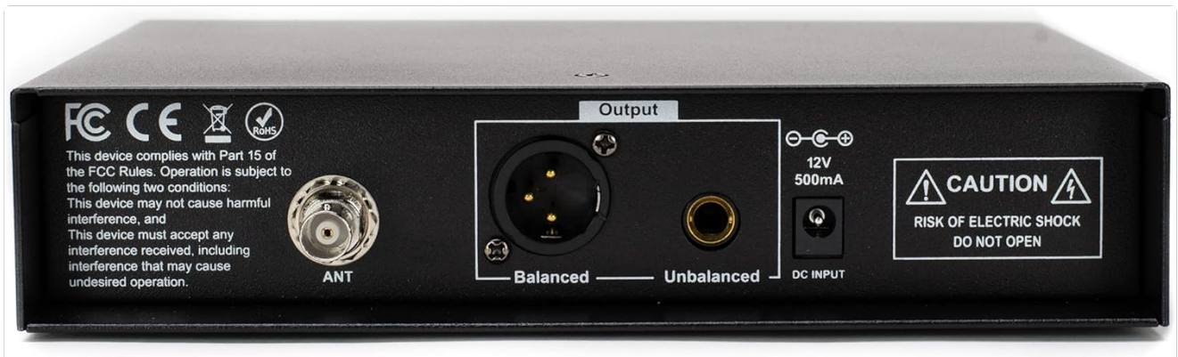
Image 3: Rear panel of the WX1000 receiver, showing the ANT connectors, Balanced XLR output, Unbalanced 1/4" TS output, and DC INPUT for power.
