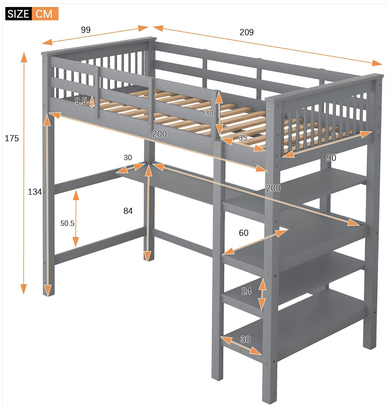
Figure 4.1: Overall dimensions of the Moimhear Loft Bed (209 x 99 x 175 cm). This diagram shows the length, width, and height of the bed, desk, and shelving units in centimeters, crucial for planning placement and assembly.
