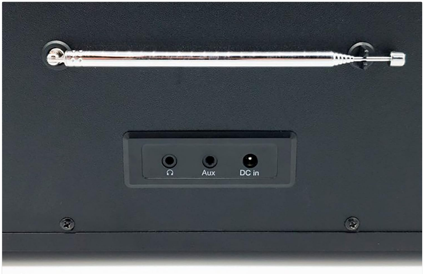
Figure 3.2: Rear panel of the unit, displaying the headphone output, AUX-IN port, and DC power input.
