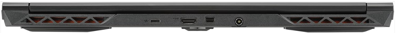
Figure 2.2: Rear view of the GIGABYTE G5 KF laptop, highlighting the power input, HDMI, Mini DisplayPort, and Thunderbolt 4 ports.
