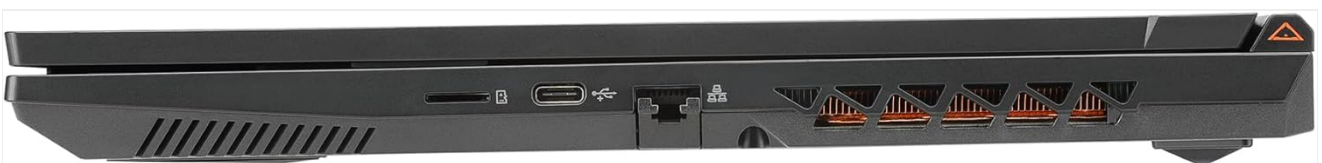
Figure 2.4: Right side view of the GIGABYTE G5 KF laptop, displaying additional USB ports and a card reader slot.
