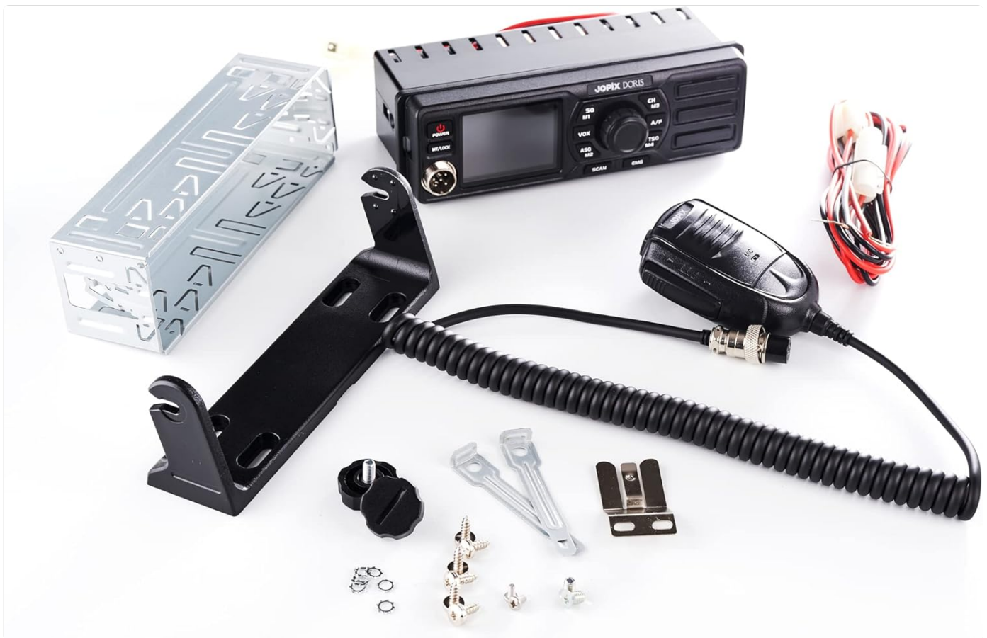
Figure 3.1: Included components of the JOPIX Doris CB Radio Station.
