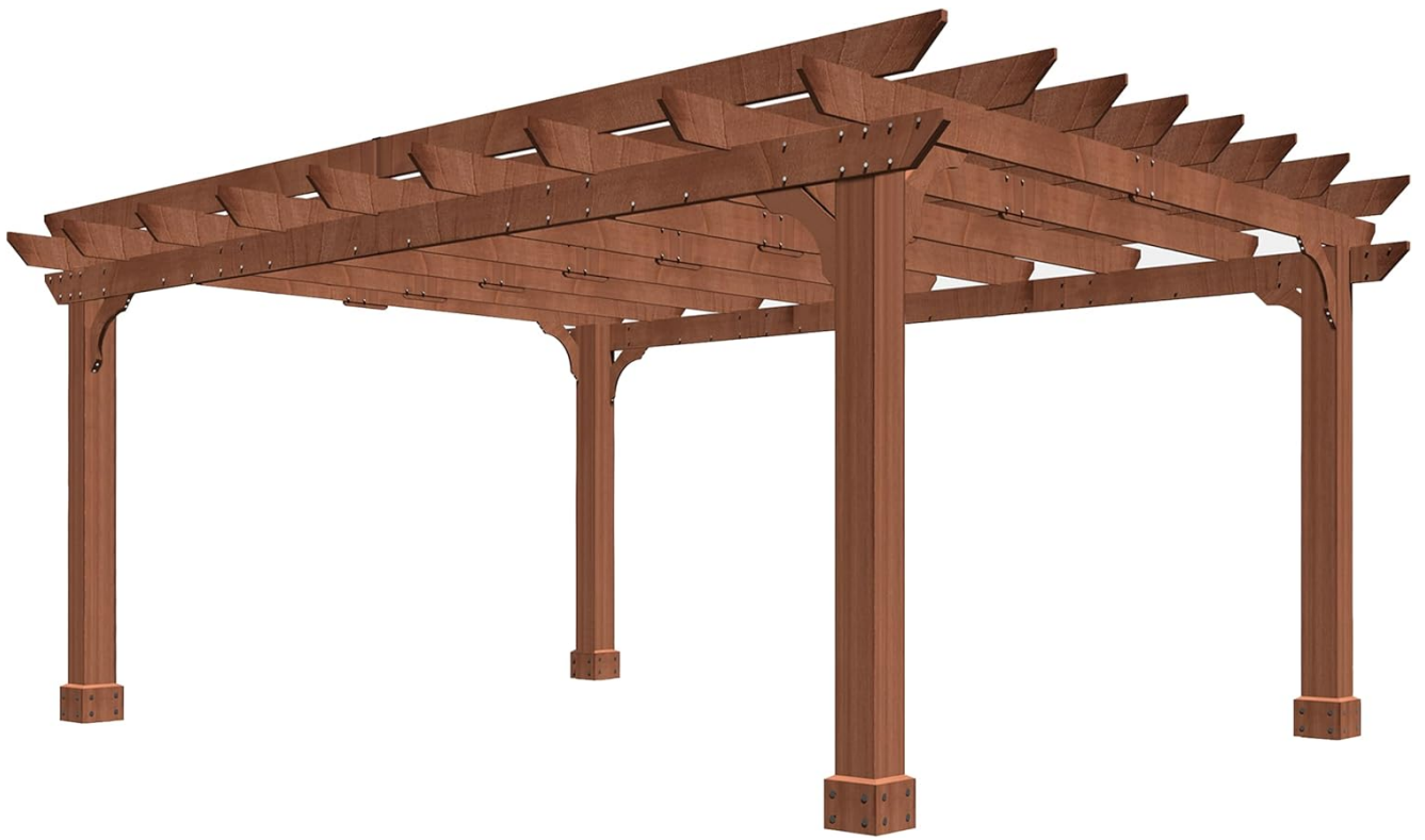
Image 5.2: Rendered view of the pergola's structural components.
