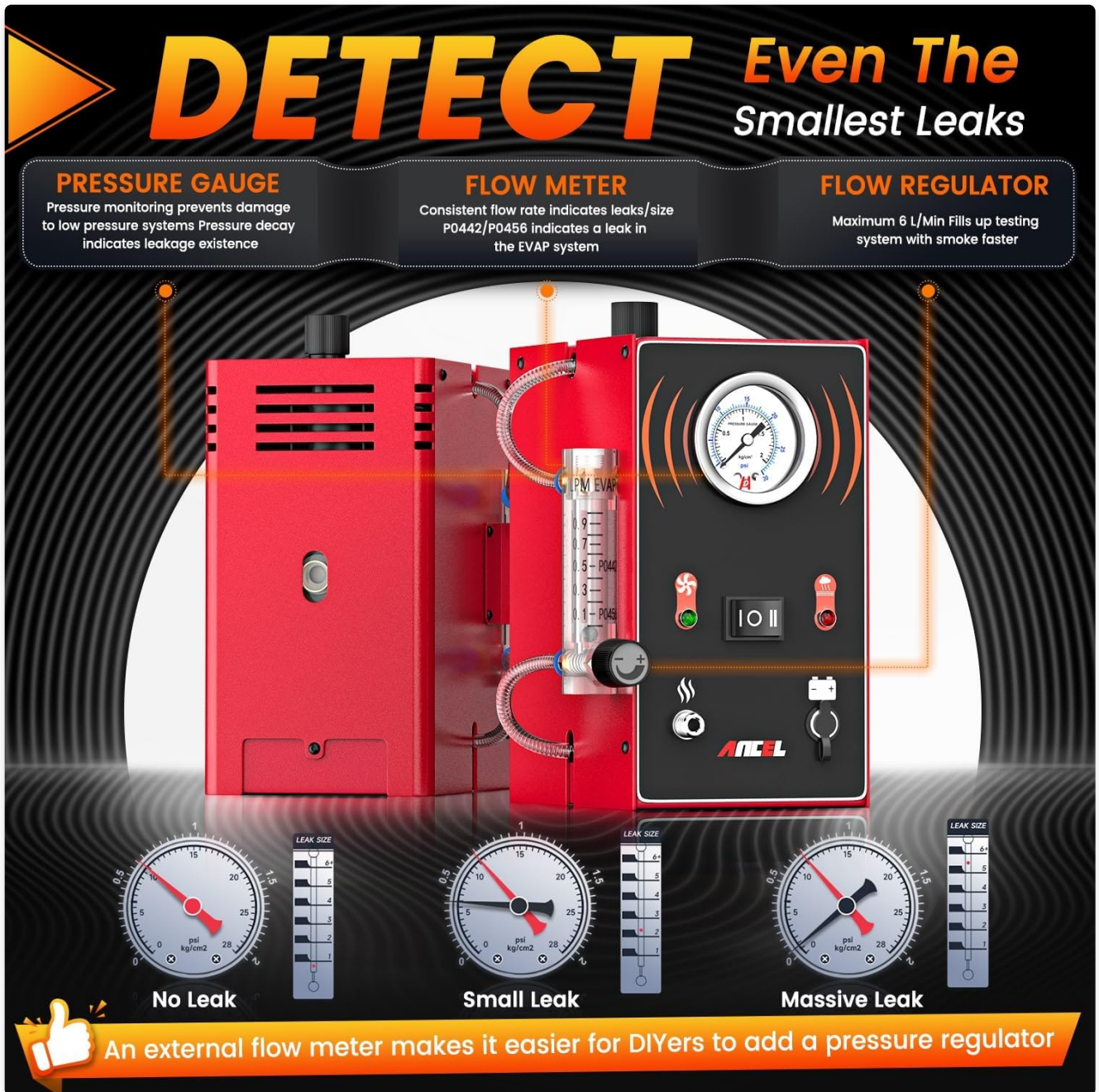
Figure 6: Understanding leak detection through pressure gauge and flow meter readings.
