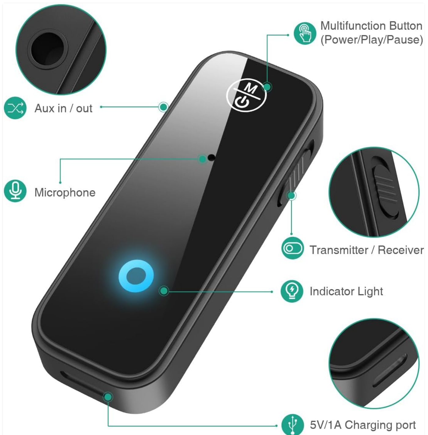
Image 2.2: Labeled diagram of the ORIA Bluetooth adapter's components. This image highlights the Multifunction Button (Power/Play/Pause), Aux in/out port, Microphone, Transmitter/Receiver (TX/RX) Mode Button, Indicator Light, and 5V/1A Charging port.
