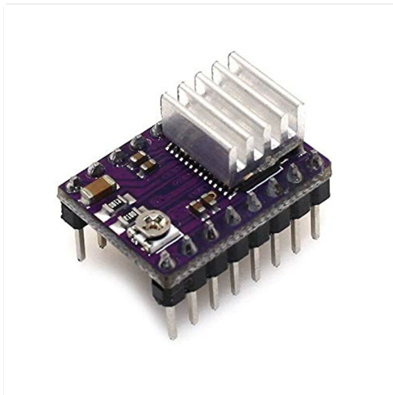
Figure 3: Individual DRV8825 stepper motor driver. This image shows a single DRV8825 driver module, highlighting its compact size and the heatsink attached for thermal management.
