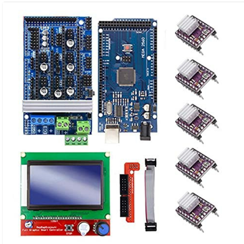
Figure 1: Overview of the Lysee Ramps 1.6 Kit components. This image displays the Ramps 1.6 control board, the Mega2560 microcontroller board, the 12864LCD graphic display, and five DRV8825 stepper motor drivers, along with connecting cables.
