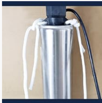
Step 3: Secure a rope or cable to the pump for lowering.
