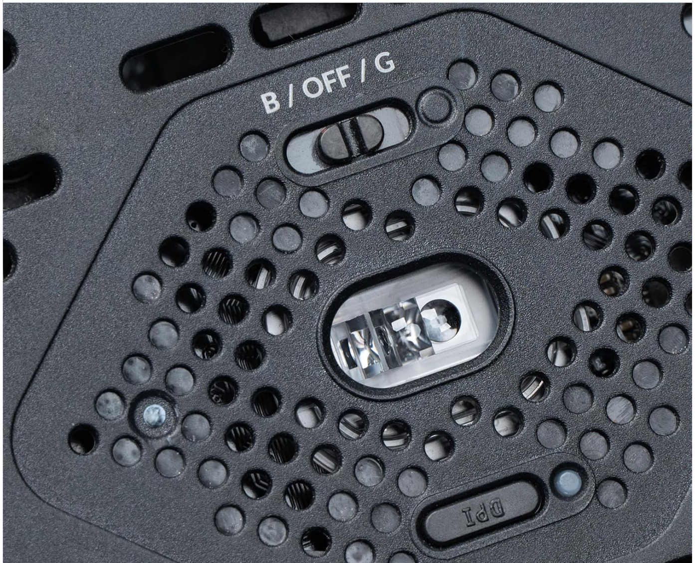
Figure 4: A close-up view of the underside of the Keychron M1 mouse, clearly showing the optical sensor, the B/OFF/G (Bluetooth/Off/2.4G) switch, and the DPI adjustment button, which allows for quick sensitivity changes up to 26,000 DPI.
