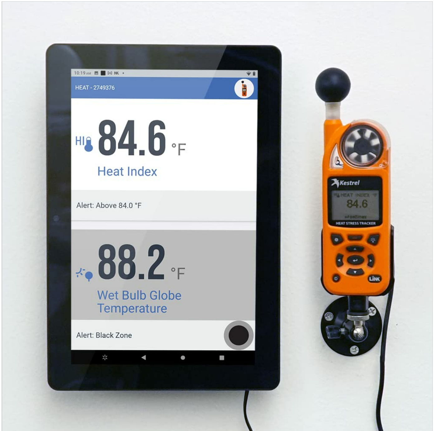
Image: The Kestrel 5400 device securely mounted on a wall, positioned beside the remote monitoring tablet, both actively displaying environmental data.
