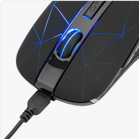
Image 6.1: The micro-USB charging port located at the front of the mouse.
