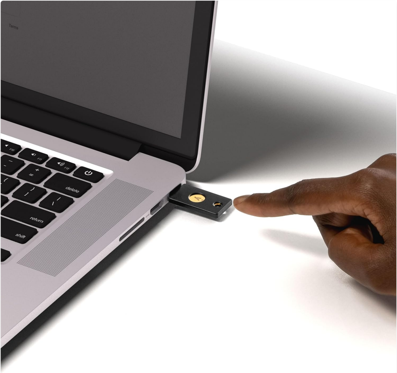
Figure 5: Demonstrates the YubiKey NFC being used with a laptop via USB-A connection.
