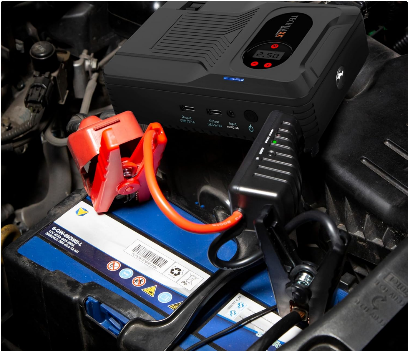
Figure 6.1: The Technaxx TX-219 connected to a vehicle battery using the provided clamps for jump starting.
