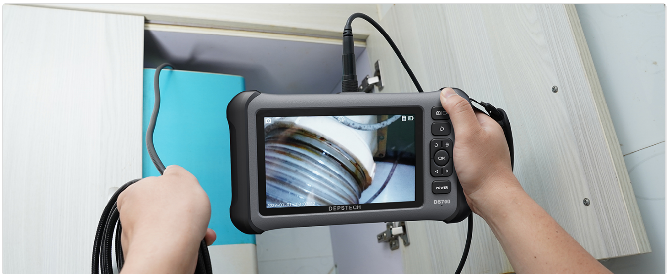
Figure 5.1: Gooseneck Cable Flexibility
