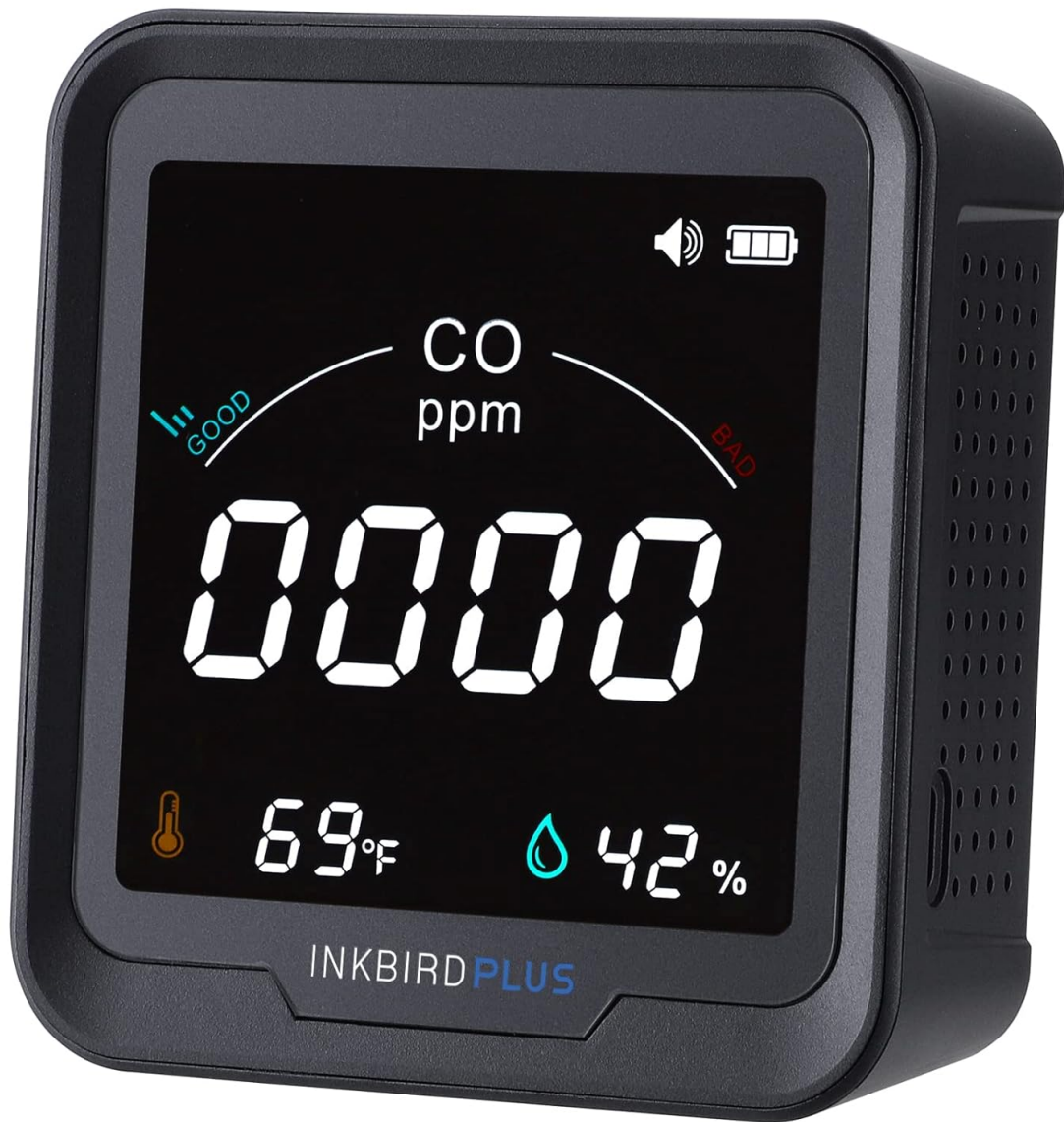
Image 4.1: The main display of the PTH-9D monitor, showing a CO reading of '0000 ppm', a temperature of 69°F, and 42% humidity, along with battery and signal indicators.
