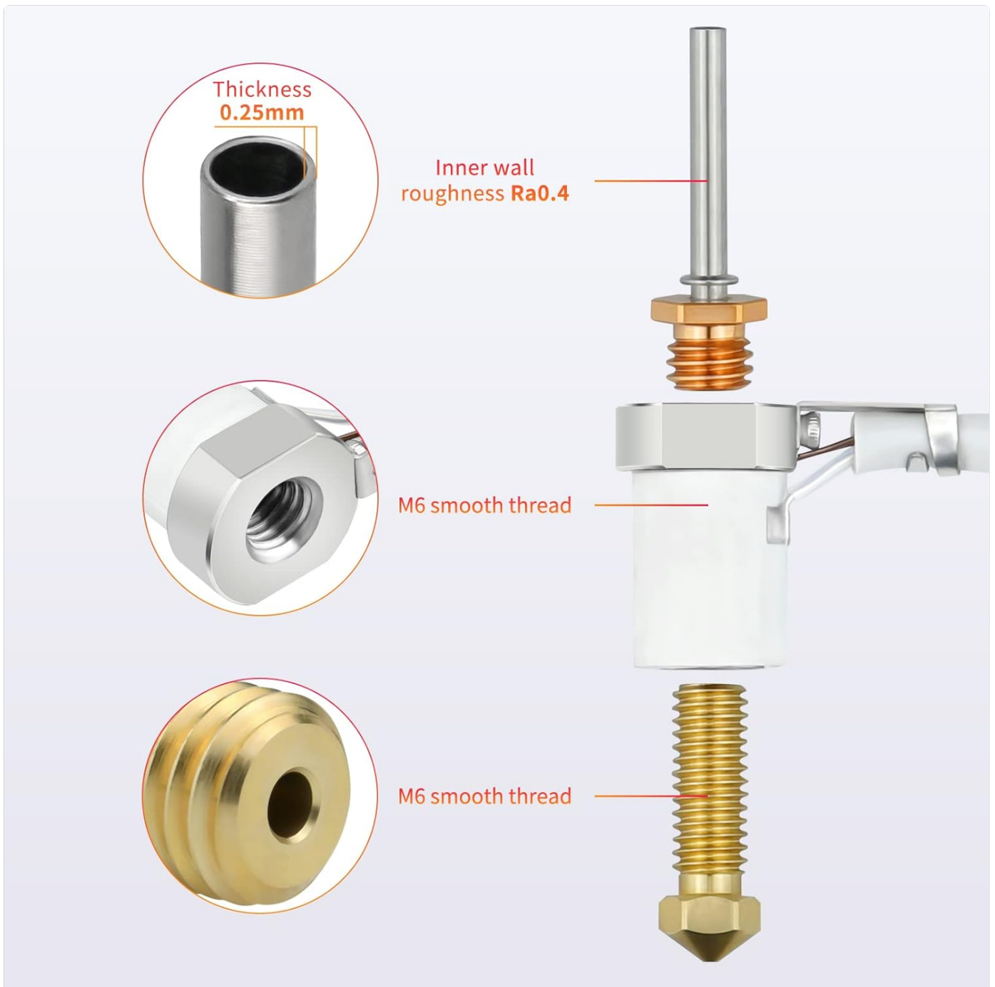
Figure 3.1: Detailed view of the heatbreak and heatblock, highlighting the 0.25mm thickness, Ra0.4 inner wall roughness, and M6 smooth threads.
