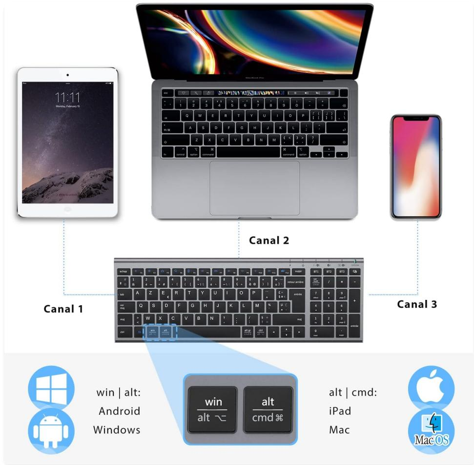
Illustration of the iClever keyboard connecting to multiple devices (iPad, MacBook, iPhone) via different Bluetooth channels (BT1, BT2, BT3). The image also highlights the automatic key mapping for Windows/Android (Win/Alt) and Mac/iPad (Alt/Cmd) systems.
