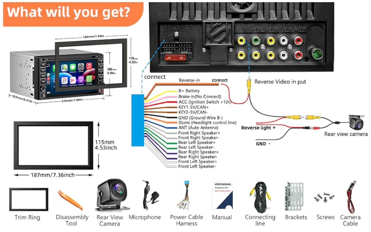
Figure 2: Illustration of package contents and a detailed wiring diagram for installation.
