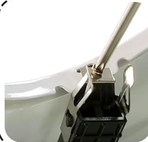
Image 4.1: Example of removing an old knob, often a preliminary step for accessing burner components.
