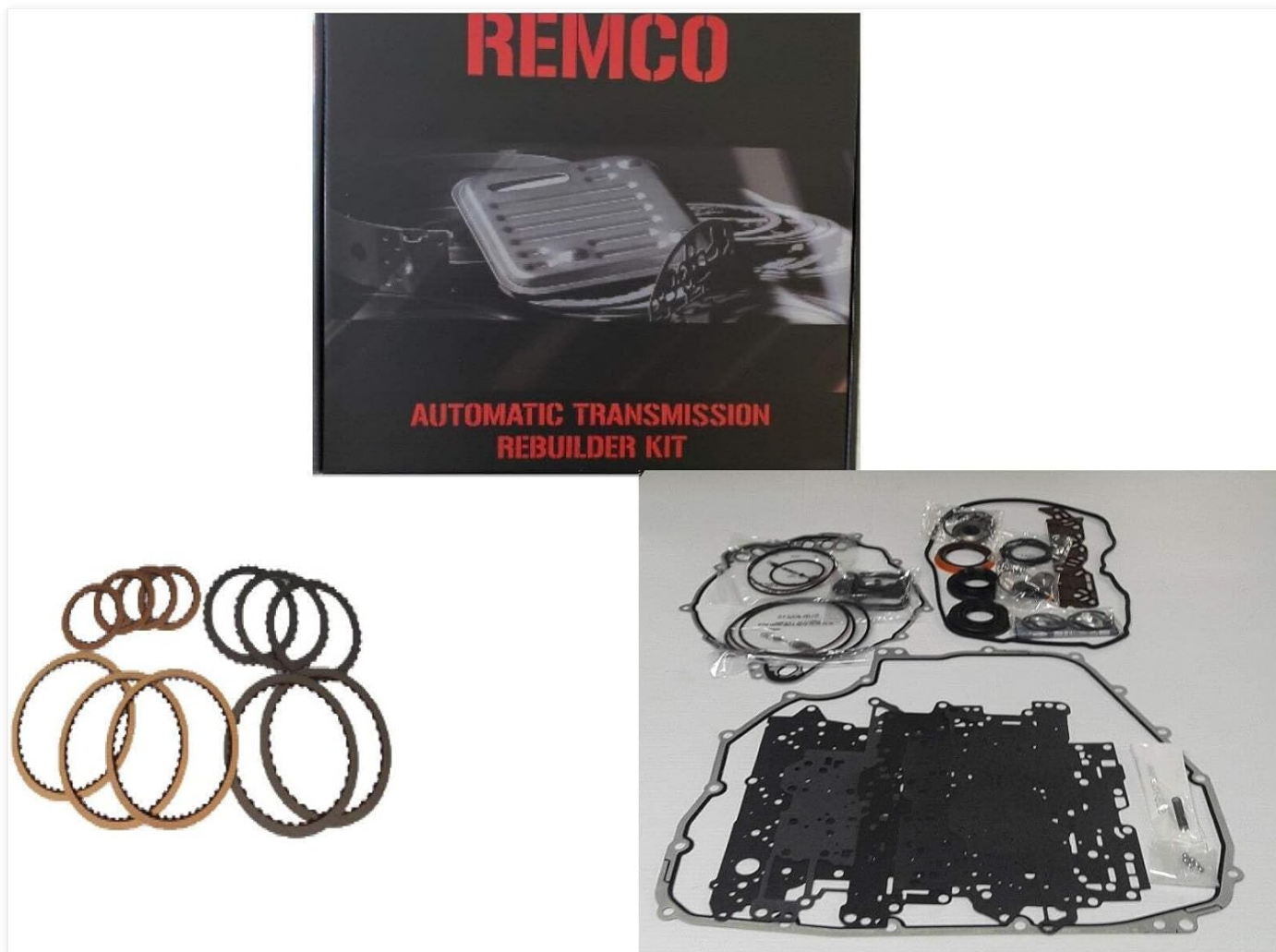
Image: Contents of the Remco 6T70 6T75E Gen 3 Transmission Banner Kit. The image displays the product packaging box, along with various components laid out, including a full set of gaskets, seals, and a collection of clutch and steel plates, essential for a complete transmission overhaul.
