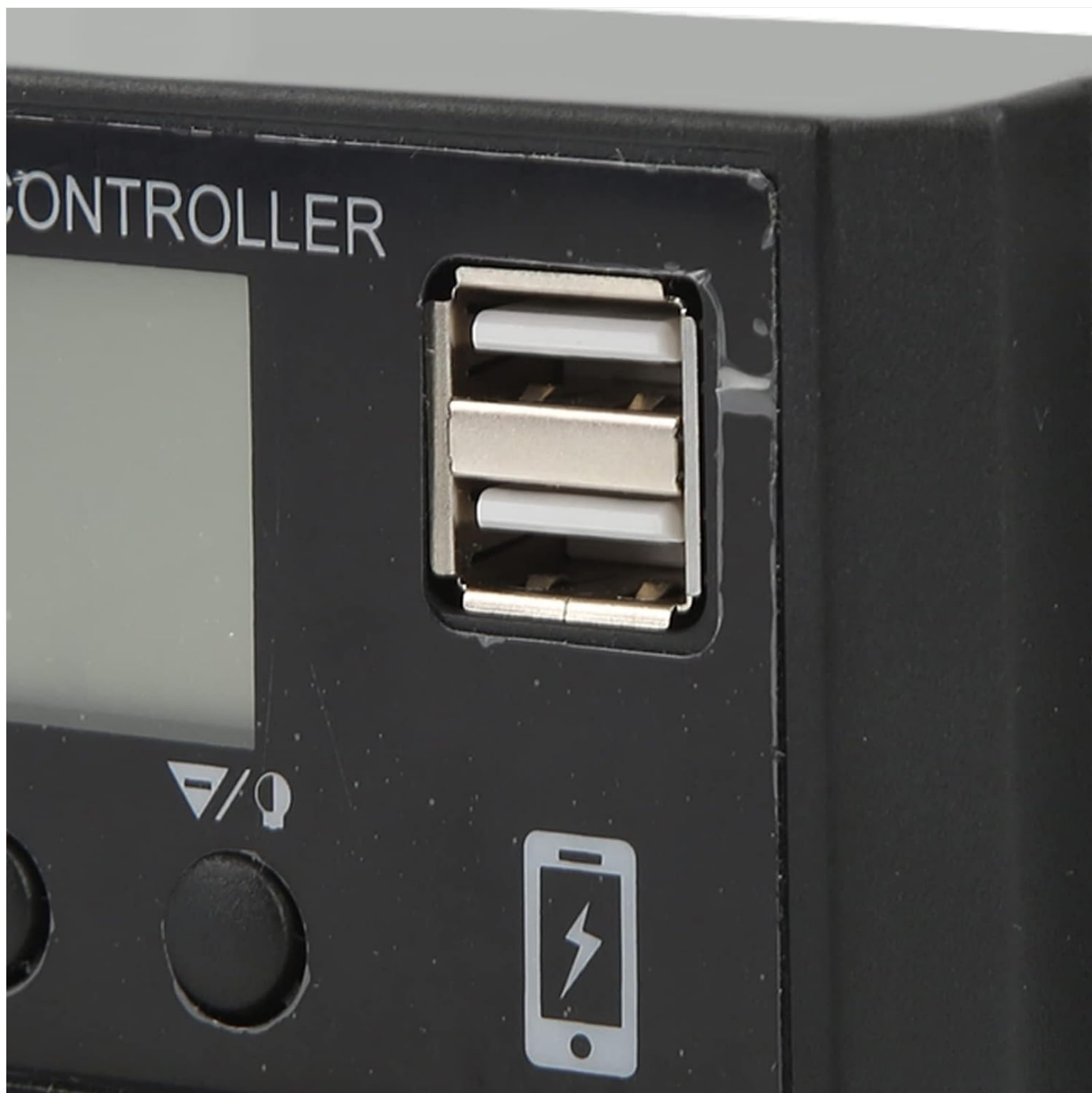
Figure 3.4: Close-up view of the dual 5V 3A USB output ports.
