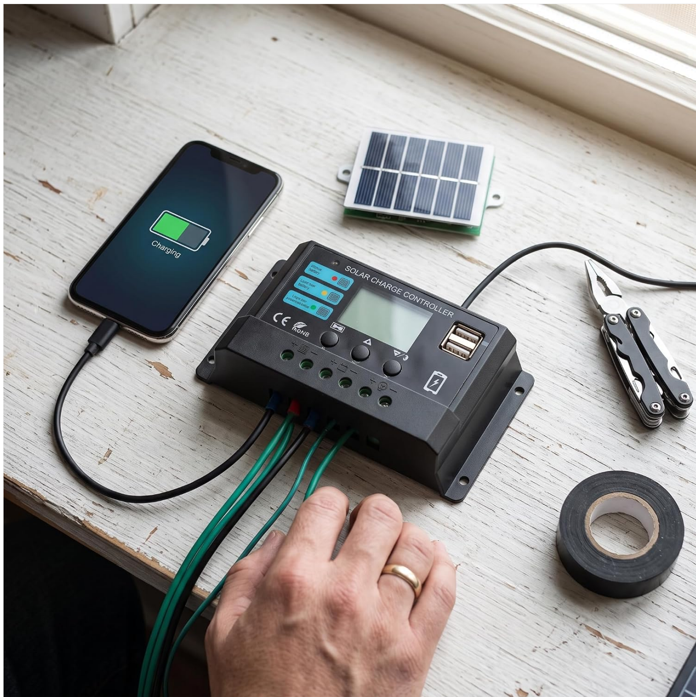
Figure 4.2: Example of the solar charge controller connected and in operation, charging a mobile device.
