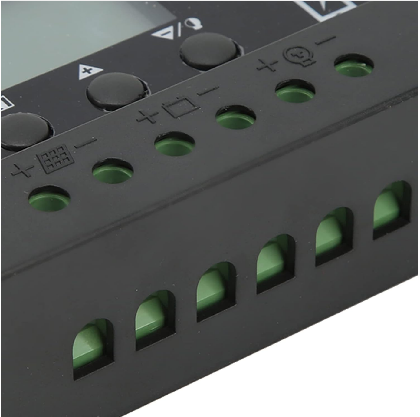
Figure 4.1: Close-up view of the wiring terminals for battery, solar panel, and load connections.
